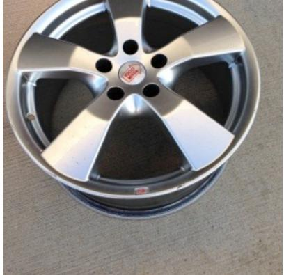
I subtract half the bead-bead distance to establish centerline at 4.0". Subtracting that from depth measure (minus 0.5 lip to bead or 5.375) I get 1.375" / 35mm. Entering into offset calculator:
